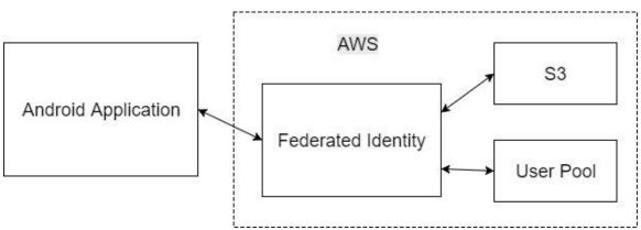
The figure above was the first initial design for our system block diagram. It has stayed the same throughout the duration of the project development time because the structure was given to us by our client. The Amazon Web Server platform and its components were already set up for the company's already existed web portal application. Because our task was to create an identical copy of their web portal application on Android, the design outside of the Android application could not be changed.
