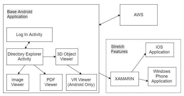
The image above is our initial proposed system event diagram. It is comprised of two key components - our Android application and AWS. AWS contains a federated identity component which is used to authorize user pools. The user pool is a group of users that are associated with our application. They will be using these services to log in and once logged in, they will have access to their data stored in AWS S<sub>3</sub>. All the client data will be viewable for the client within the application.
